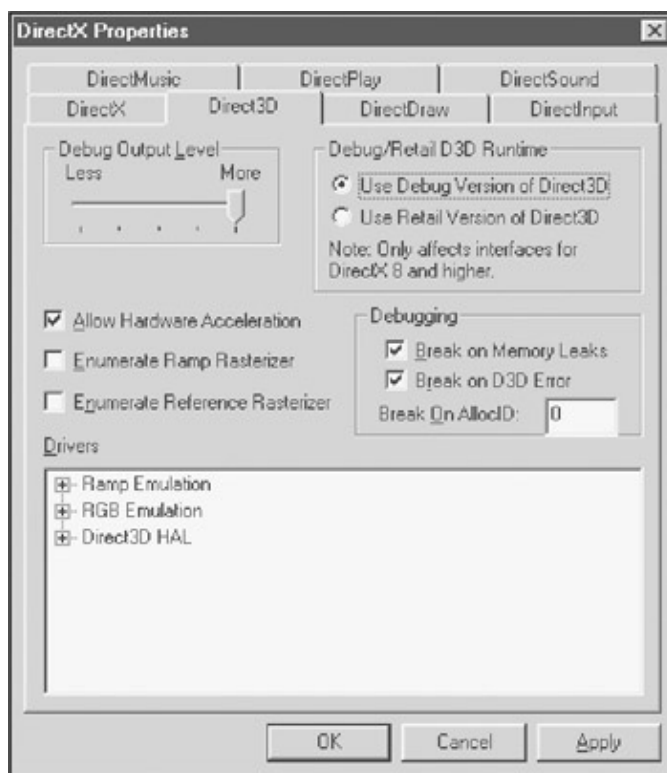
Figure 1.3: The DirectX system properties give you a multitude of options. In this case, the Direct3D tab has been selected, and you can see that the debug libraries are in use at the highest debug output level.
