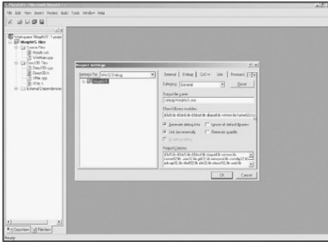
Figure 1.6: The Project Settings Link properties allow you to specify exactly which library files to link to your application.
