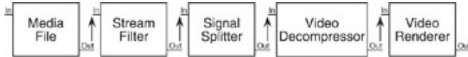
Figure 14.3: A sample set of four filters is used to grab data from the media file, decode it, and finally render it to the video display
